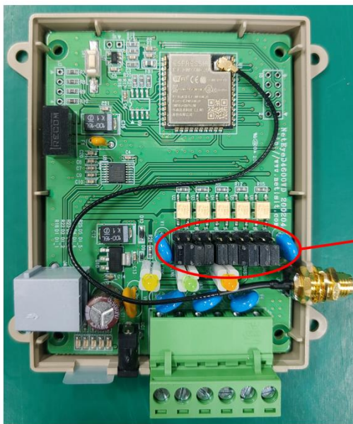
[Dry mode Switch configuration]
